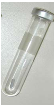
2-5 mL Round bottom reactor tube
