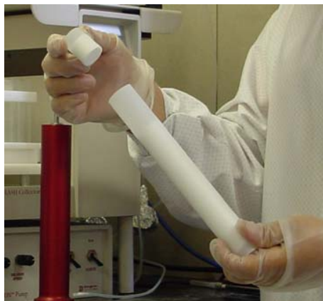
Figure 2: Samplet containing product is inserted onto Flash 25+™M cartridge
