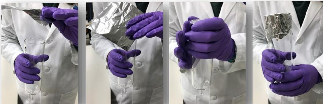
**Step 4:** Slide the covered evaporation tube into the evaporator, making sure the edges of the tinfoil are trapped along the sides of the tubes.
