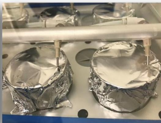
**Step 6:** Open the lid and puncture larger holes, approximately 1 cm in diameter (or the width of most ballpoint pens). Use the marks in the tin foil as your guide.
