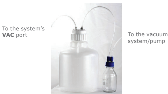
Figure 25. The waste & scrubber kit contains a 10 liter waste reservoir, a 0.5 liter scrubber bottle, and the tubing shown above.
