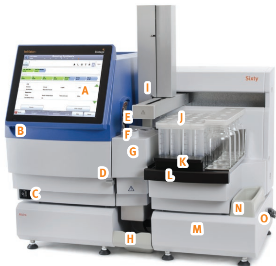
Figure 18. A = touch screen, B = USB port, C = mains switch, D = vial eject lever, E = microwave cavity and needle wash station (behind the cavity), F = holder for the vial collar, G = cavity cover, H = waste tray, I = robot arm with dispensing needles, J = cover plate, K = amino acid rack, L = rack tray for amino acid rack(s) and reagent bottles, M = Alstra pump module, N = accessories holder, and O = solvent inlets, and
