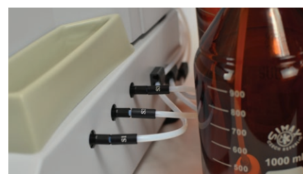
Figure 24. Three solvent inlets are available on the right hand side of the system.
