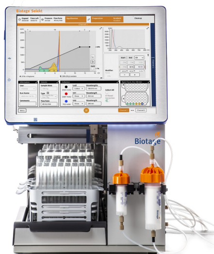
Figure 2. Biotage® Selekt Enkel with remote access and monitor API
