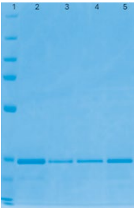
FIGURE 2: Consistency yields for Ni-IMAC resin with 40uL volume, tested on 300mg of His-eGFP protein for each respective protein purification platform at standard conditions.
