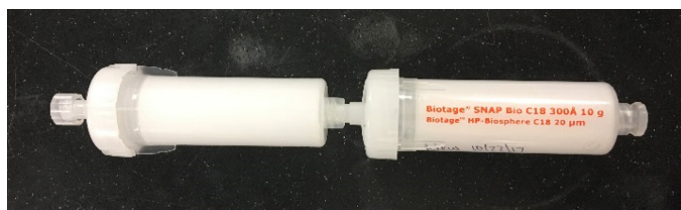
Figure 8. Rather than constructing a whole new column, two Biotage® SNAP cartridges can be connected via the outlet and inlet luer fittings.
