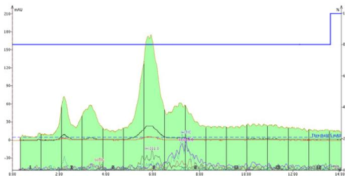
Figure 4. Isocratic purification of natural CBN created through THC oxidation. CBN is the large peak at 5 minutes with a detected mass of +311. THC elutes just after CBN and has a detected mass of +315.
