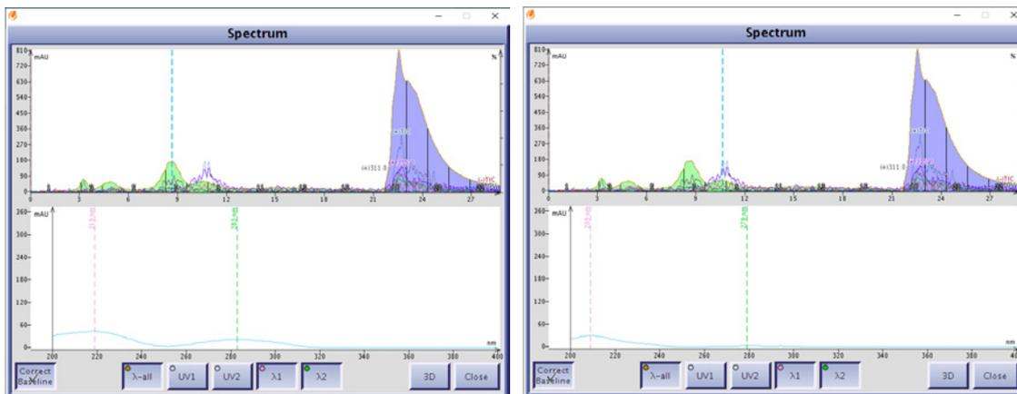
Figure 5. Purified degraded THC extract UV spectra identifies the tall green peak as CBN with UV maxima at 218 nm and 283 nm (left) and the adjacent peak to the right as THC with UV maxima of 209 nm and 278 nm (right).
