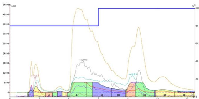
**Figure 1.** Simple step gradient purification method for synthetic CBN using both UV and mass detection. CBN is the big peak in the middle with a detected negative ionization mass of -309.
