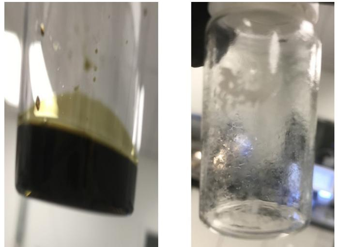
**Figure 6.** Before and after flash chromatography photos shows the crude CBN reaction mixture (left) and purified CBN (right).
