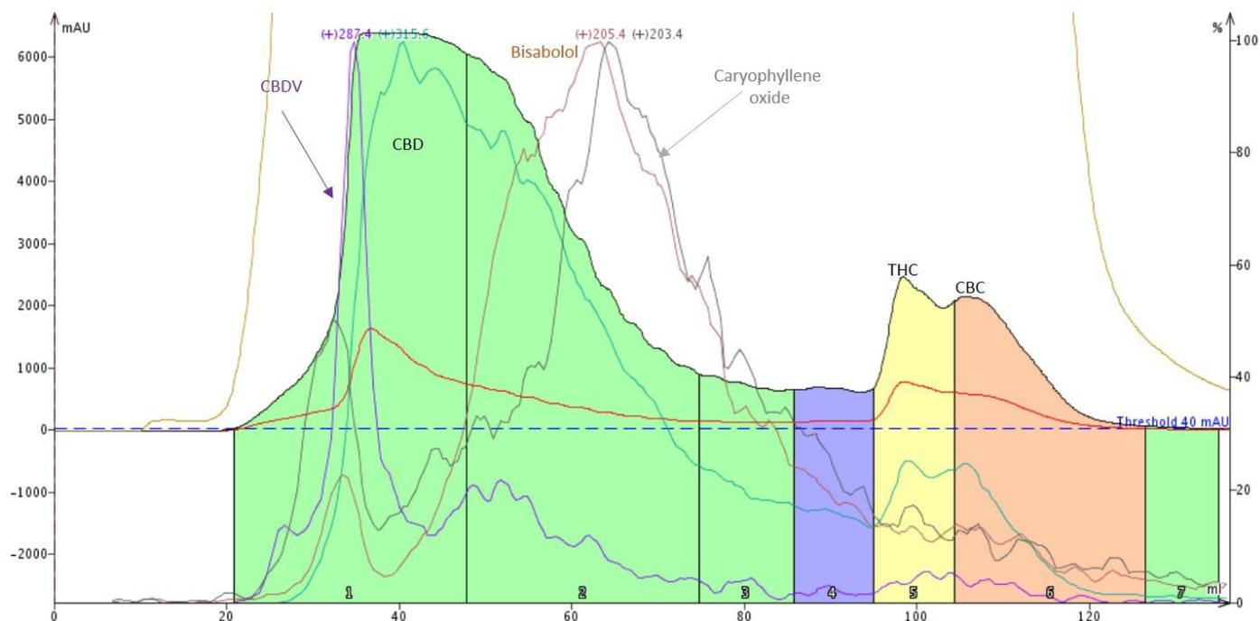
**Figure 1.** Hemp extract (800 mg load) containing ~2.5% THC and ~75% CBD purified using a 12-gram Biotage® Sfär C18 flash chromatography column and a Biotage® Isolera Dalton 2000 system. The green peak is CBD, the yellow peak is THC and the orange peak is CBC. Also removed from THC are CBDV (purple trace) and two terpenoids, bisabolol (rust trace) and caryophyllene oxide (gray trace). Along with UV, an optional inline mass detector was used to verify compound identification.
