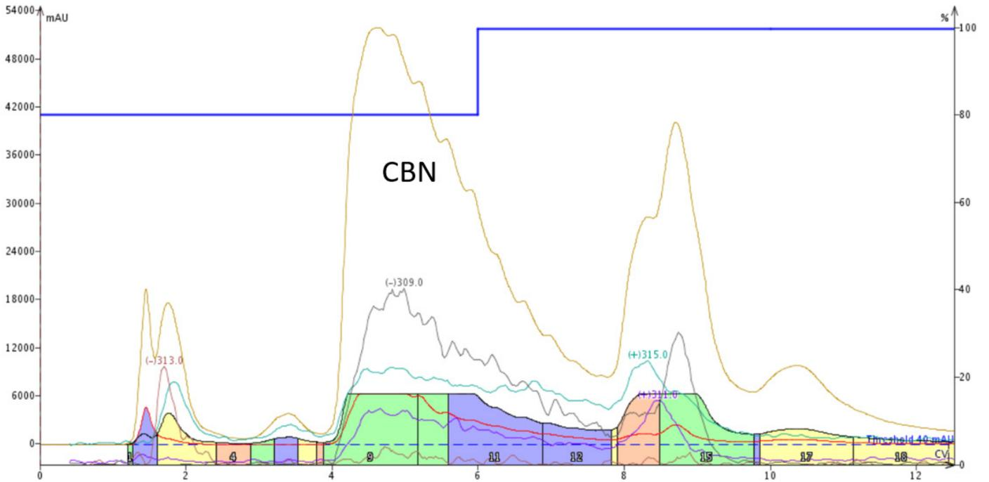
**Figure 4.** CBN purification using reversed-phase flash chromatography. CBN is easily separated from this reaction mixture's by-products. The optional in-line mass detector confirmed CBN's identity with a detected mass/charge ratio of 309.
