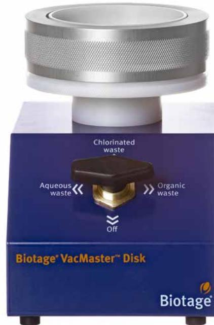
8. Elute the SPE Disk: (Please note: the elution solvent will go into the collection flask inside the chamber, not to waste containers; omit multifunnel steps if not using)
