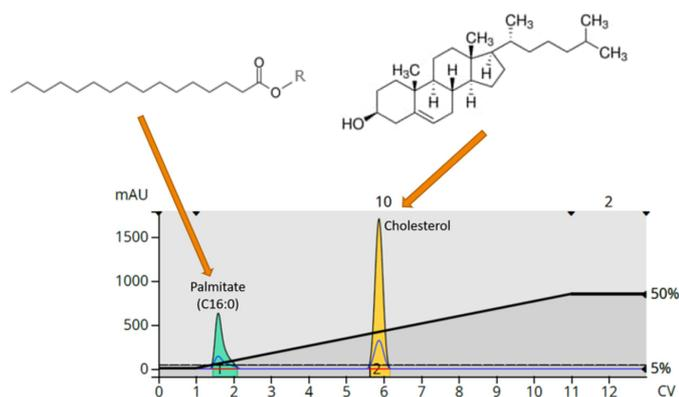
**Figure 1.** Normal-phase flash chromatographic purification of methyl palmitate and cholesterol. The fully saturated palmitate is too lipophilic to be retained on the normal phase stationary phase, while cholesterol, with its hydroxyl group, is well retained, and elutes later in the run.
