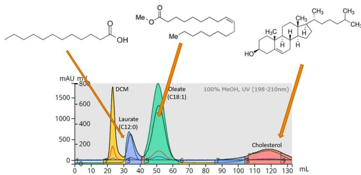
**Figure 2.** Reversed-phase flash chromatography purification of methyl laurate, methyl oleate, and cholesterol in 100% methanol with UV (198–210 nm). This example shows the application of ELSD detection. These lipids are easily detected by both UV and ELSD including the fully saturated methyl laurate.
