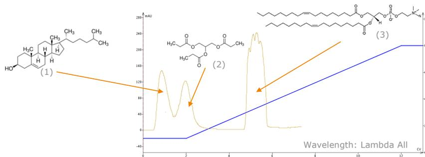
**Figure 3.** Normal phase flash chromatography purification of Cholesterol, Tripionin, DOPC in hexane / ethanol showing the effect of powerful lambda all.
