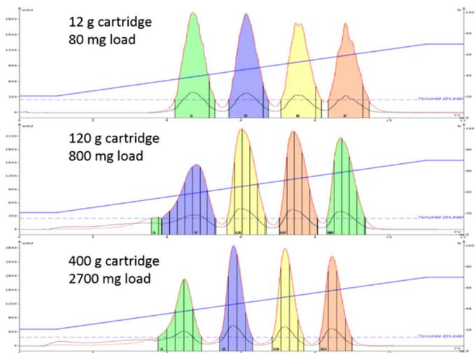
**Figure 4.** An example of scale up theory. If a 10g development cartridge has a scale factor of 1, then a 50 g cartridge has a factor of 5, a 400 g cartridge has a scale factor of 40 and thus a 40 Kg cartridge has a factor of 4000. Using the same stationary phase in our development, we have identical chemical selectivity and retention on scale up, meaning predictable compound elution. Therefore, small scale is seamlessly transferred to large multi-Kg scale.
