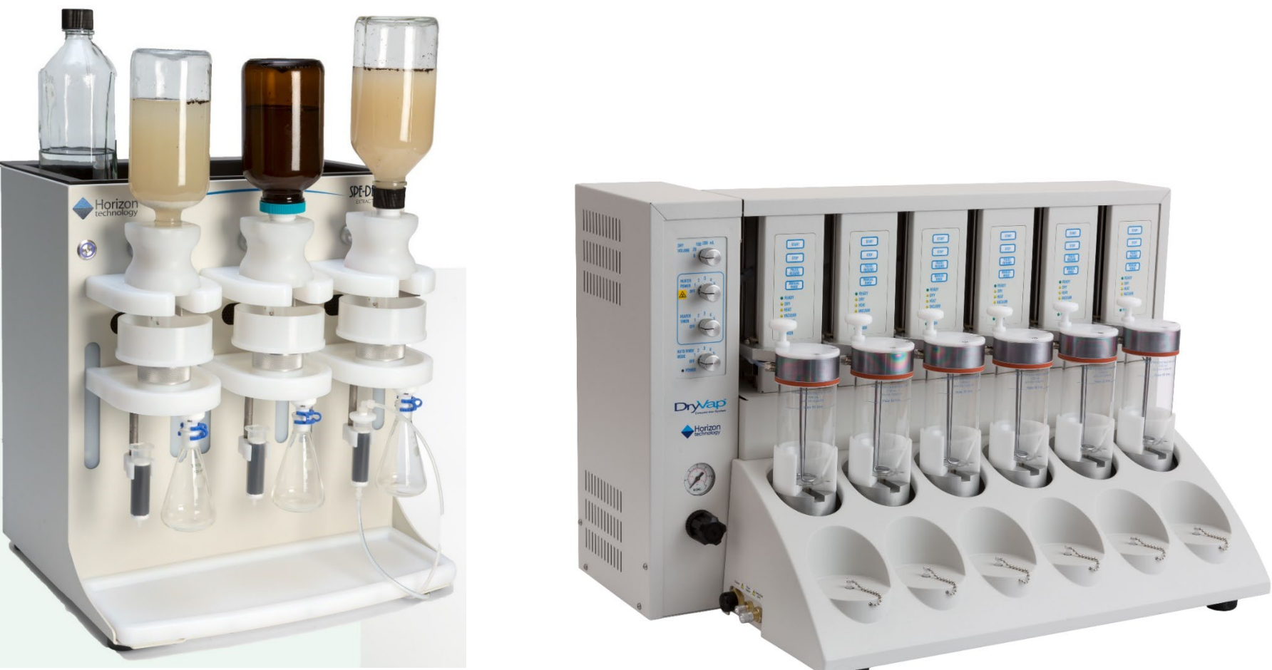
Figure 1. Extraction and drying systems used for sample preparation: the Biotage® Horizon 5000 (previously known as the SPE-DEX 5000) (left) and the DryVap™ System (right).
