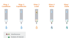
Figure 2. Schematic of a Typical SPE Procedure.
