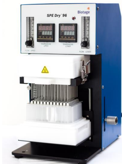
Figure 3. Biotage® SPE Dry 96 Plate Evaporator, P/N SD-9600-DHS-NA with ACT Plate Adapter
