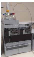
Figure 1. Nexera UHPLC with reduced PFAS tubing.
