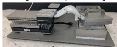
Figure 2. Cleavage transfer unit transfers cleaved peptide solution from 96 syringe-like reactor vials into a deep-well 96-well plate simultaneously.
