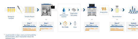
Figure 2. Biotage ISOLUTE® SLE+ automation workflow for sample preparation in Bioanalysis
