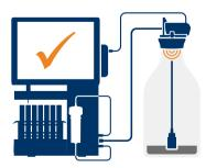
When the waste level is at 95% of the set capacity, the run is automatically paused and the user will be prompted to empty the waste reservoir.
