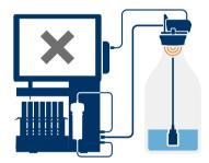
When the solvent surface is 30 mm from the bottom of the reservoir, the run is automatically paused and the user will be prompted to refill the solvent reservoir.
