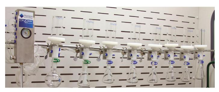
The DryDisk® membrane drying system provides advantages for removing water from nonpolar solvents, important in protecting the chromatograph in the analysis step, especially critical in protecting GC and GC/MS.
