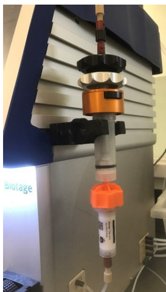
Figure 4. External dry loading uses dried mixture of crude with a solid support media packed into a column mounted on top of the primary purification column.
