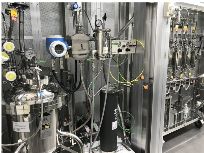
Fig 1. Purification system adapted for HPAPI handling with Biotage® Flash 150 system as the core. The system fits inside a draft and was designed by an engineering company.
