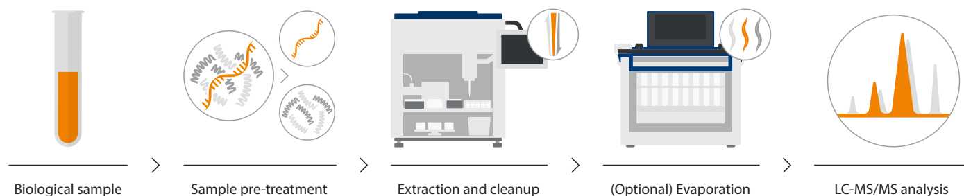
Figure 3. Biotage® Oligo SPE end-to-end workflow for bioanalytical sample preparation, with the integration of pre-treatment, extraction, clean-up, and evaporation steps.
