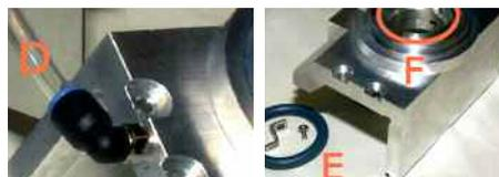
VI. Clean the cavity lid seal with water or alcohol containing mild soap. Do not use aromatic or chlorinated solvents.
