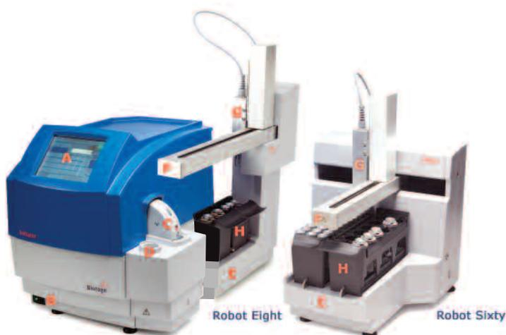
A = touch screen, B = main switch, C = cavity lid, D = cavity insert located in the insert holder, E = robot, F = sampler arm, G = gripper and H = rack.
