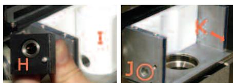
XIII. Remove the cavity air guide (I) and clean it using a cloth. If the cavity air guide is broken or distorted, replace it.
