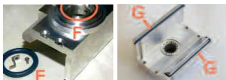
X. Put the cavity lid seal back in place.
