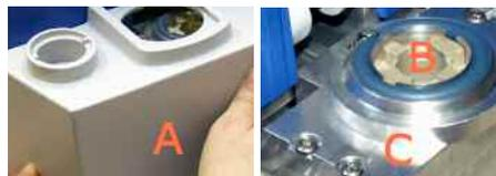
IV. Remove the service lid (C) by undoing the four screws and disconnecting the air tubing (D). Push in the blue collect against the black fitting and pull the tubing out.
